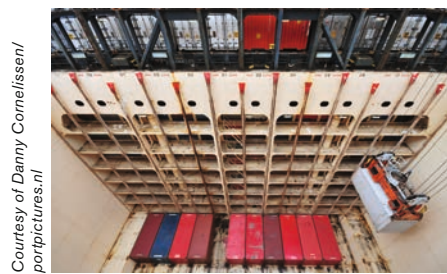
Figure 41.20: 1990s 4,500 TEU cellular container ship.
