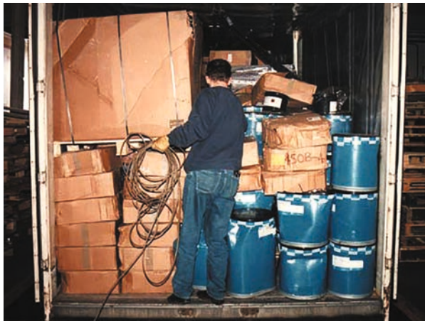
Figure 41.3: Poorly stuffed container – note the damaged packages, the pallet on top of cartons and the apparent lack of securing arrangements.
