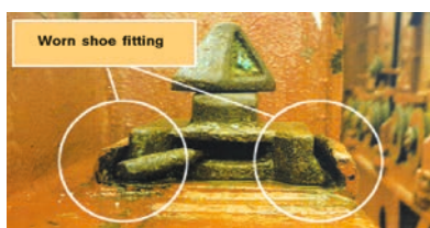
Figure 41.12: Worn shoe fitting.
