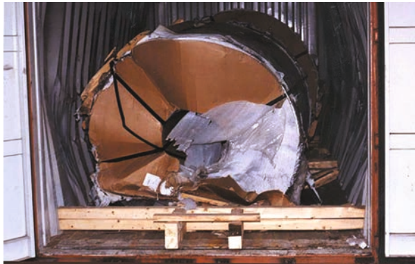
Figure 41.5: Damage caused to a container by poorly secured coils.
