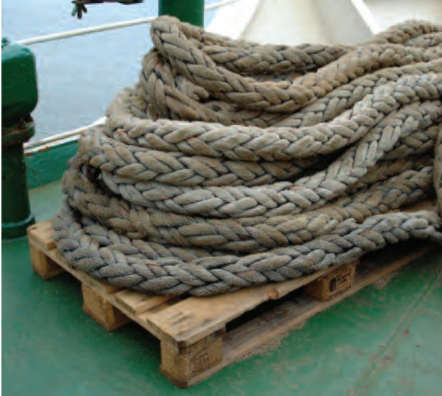
Ropes correctly stowed off deck
