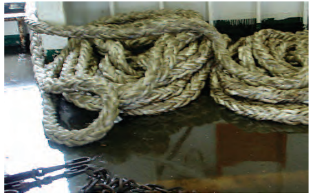
Ropes badly stored on wet deck
