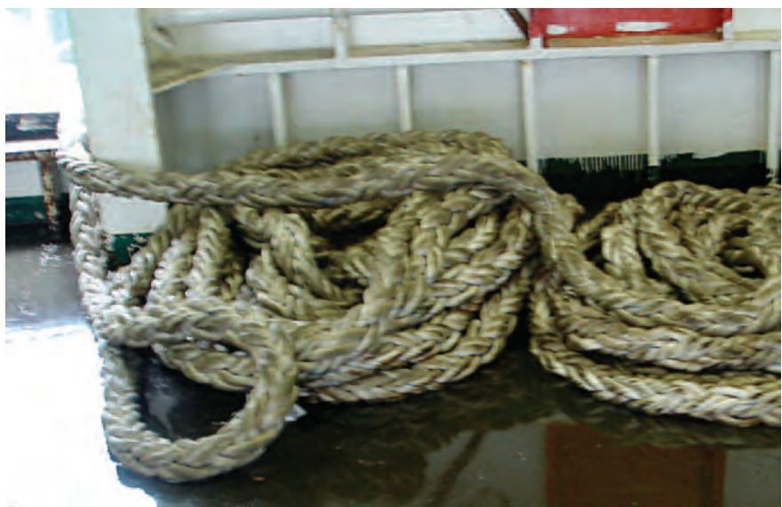
Ropes badly stored on wet deck
