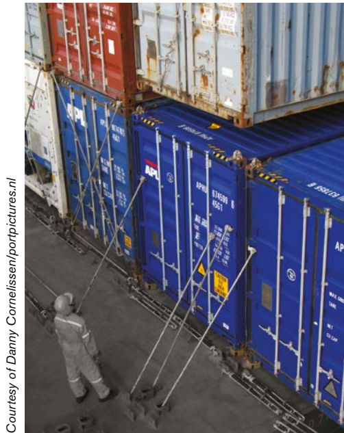
Figure 41.17: The safe lashing of containers.
