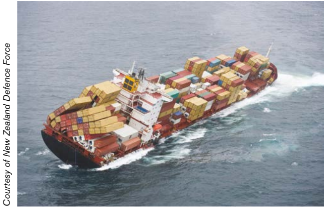
Figure 41.1: The grounding of MV 'Rena' off New Zealand in 2011 overstressed many container twistlocks, resulting in a partial collapse of container stacks.
